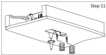
**Step 11** - Remove Fixture Ring and Connect LED Light: a. Insert Ring Clip and Turn Counterclockwise to remove LED Ring Holder. b. Connect LED Light and insert through Fixture and replace Ring.
