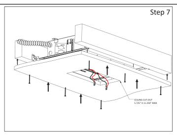
**Step 7 -** Cut-Out Dry-wall and Install to Ceiling Joist: a. Mark the Fixture location on Dry-wall "Sheet" and cut-out.
