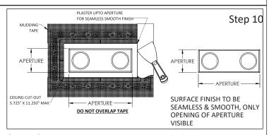
Step 10 - Plastering Ceiling Cut-Out with fixture and Paint
