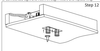
**Step 12** - Replace Fixture Ring and Install LED Light: a. Insert LED Light and Turn Clockwise Fixture Ring to hold LED.
