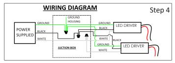
Step 4 - Connect Power Supply to Fixture J-Box:
