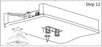
**Step 12** - Replace Fixture Ring and Install LED Light: a. Insert LED Light and Turn Clockwise Fixture Ring to hold LED. b. Aim led to desired area.
