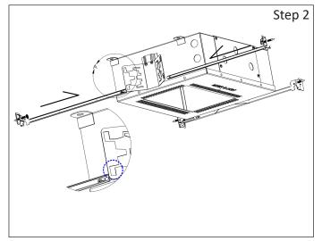
**Step 2** - Install hanger bars to Fixture: a. Align the hanger bars to the outside rectangular holes of butter fly bracket; indicated by dash cirlce. (Provided).
