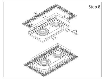
**Step 8** - Harmony trim assembly: a. Assemble Harmony trim with mesh by aligning hole of mesh and
