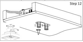
**Step 12** - Replace Fixture Ring and Install LED Light: a. Insert LED Light and Turn Clockwise Fixture Ring to hold LED. b. Aim led to desired area.
