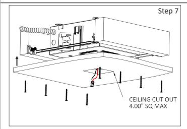
**Step 7** - Cut-Out Dry-wall and Install to Ceiling Joist: a. Mark the Fixture location on Dry-wall "Sheet" and cut-out. b. Slide Fixture through butterfly brackets to Center the Ceiling Cut-out and Lock position using screw (provided). c. Align the Cut-out with Fixture.
