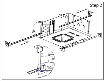
**Step 2** - Install hanger bars to Fixture: a. Align the hanger bars to the outside rectangular holes of butter fly bracket; indicated by dash cicrle. (Provided).
