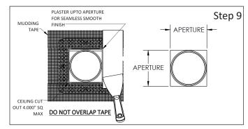
**Step 9** - Plastering Ceiling Cut-Out with fixture and Paint: a. Apply mudding tape joining ONLY the outerlip of the fixture to cover the drywall <u>DO NOT OVERLAP TAPE.</u>
