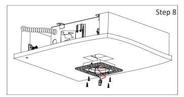
**Step 8** - Attach Boost trim to Fixture: a. Align Boost trim assembly and insert in the Cut-out. b. Secure Boost trim assembly with plaster/sheetmetal screws((4) By others)
