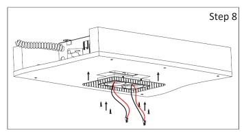
**Step 8** - Attach Boost trim to Fixture: a. Align Boost trim assembly and insert in the Cut-out. b. Secure Boost trim assembly with plaster/sheetmetal screws((4) By others)
