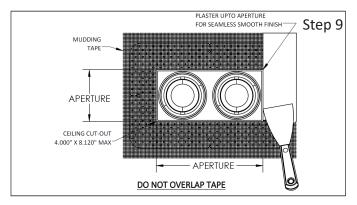
**Step 9** - Plastering Ceiling Cut-Out with fixture and Paint: a. Apply mudding tape joining ONLY the outerlip of the fixture to cover the drywall <u>DO NOT OVERLAP TAPE.</u>
