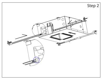
Step 2 - Install hanger bars to Fixture: a. Align the hanger bars to the outside rectangular holes of butter fly bracket; indicated by dash cirlce. (Provided).
