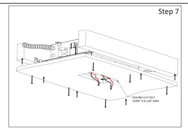
**Step 7 -** Cut-Out Dry-wall and Install to Ceiling Joist: a. Mark the Fixture location on Dry-wall "Sheet" and cut-out. b. Align the Cut-out with Fixture and secure drywall.
