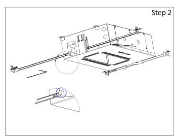
Step 2 - Install hanger bars to Fixture:
