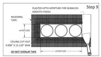
**Step 9** - Plastering Ceiling Cut-Out with fixture and Paint: a. Apply mudding tape joining ONLY the outerlip of the fixture to cover the drywall **DO NOT OVERLAP TAPE.**
