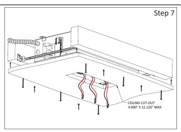
Step 7 - Cut-Out Dry-wall and Install to Ceiling Joist:
