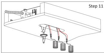
**Step 11** - Remove Fixture Ring and Connect LED Light: a. Insert Ring Clip and Turn Counterclockwise to remove LED Ring Holder.
