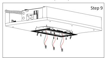
**Step 9** - Attach Harmony trim to Fixture: a. Align Harmony trim assembly and insert in the Cut-out.
