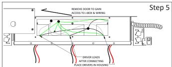
**Step 5** - Install the Driver: a. Remove j-box cover plate and attached conduit with line voltage to fixture.
