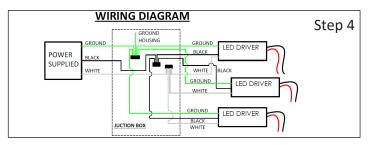
Step 4 - Connect Power Supply to Fixture J-Box:
