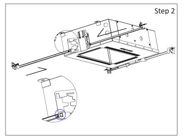
**Step 2** - Install hanger bars to Fixture: a. Align the hanger bars to the outside rectangular holes of butter fly bracket; indicated by dash circle. (Provided).
