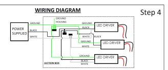
Step 4 - Connect Power Supply to Fixture J-Box:a. Connect Power Supply using Conduit Fitting (By Others) to J-Box.b. Pull out Supply Wires and make Wiring Connections, see Wire Diagram.
