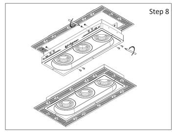
**Step 8** - Harmony trim assembly: a. Assemble Harmony trim with mesh by aligning hole of mesh and Harmony trim
