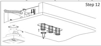
**Step 12** - Replace Fixture Ring and Install LED Light: a. Insert LED Light and Turn Clockwise Fixture Ring to hold LED. b. Aim led to desired area.
