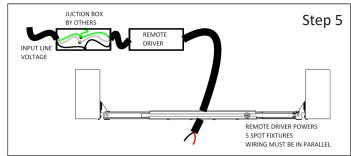
**Step 5** - Run led connection to 5 Spot fixtures:
