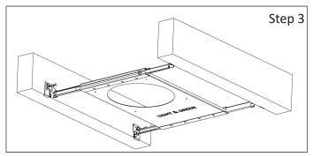
Step 3 - Install Fixture Assembly to Wood-Joist:
