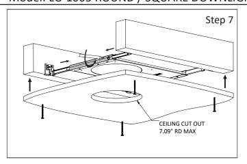
Step 7 - Cut-Out Dry-wall and Install to Ceiling Joist:
