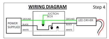
**Step 4** - Connect Power Supply to remote driver/J-Box:
