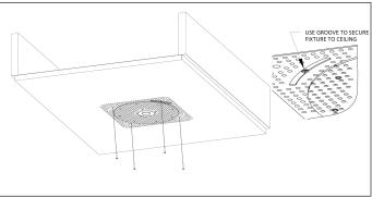
**Step 8** - Attach Spot fixture to ceiling: a. Align Spot trim assembly and insert in the Cut-out. b. Secure Spot trim assembly with plaster/sheetmetal screws(4) through groove slots.
