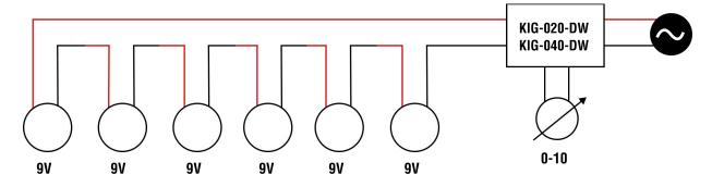
KIG-020-DW carries a load of 1-4 fixtures KIG-040-DW carries a load of 1-7 fixtures
